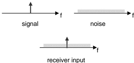
The noise power density is more or less flat over the entire frequency range, but there may also be some peaks from specific sources. There are multiple sources of noise: Radiation from nearby electronic devices that is coupled into the antennas, radiation from the on board digital electronics that is coupled into the antennas, crosstalk between digital and analog signals on the printed circuit and noise caused by receiver circuits etc.
