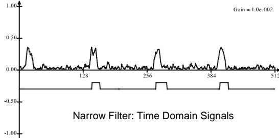
Also, the impulse rise time is now much longer because of the reduced filter bandwidth. It is not possible any more to properly characterize an impulse because of the time limit imposed by the 70 ms minimum pulse duration as specified in EN 300 718.
