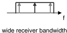
A restriction of the transmitter frequency tolerance to  $\pm 50$  Hz can be achieved at no extra cost by proper quartz crystal selection and oscillator circuit design. Widening the receiver filters affects the SNR (Signal to Noise Ratio), which is the most important parameter for receiver performance.
